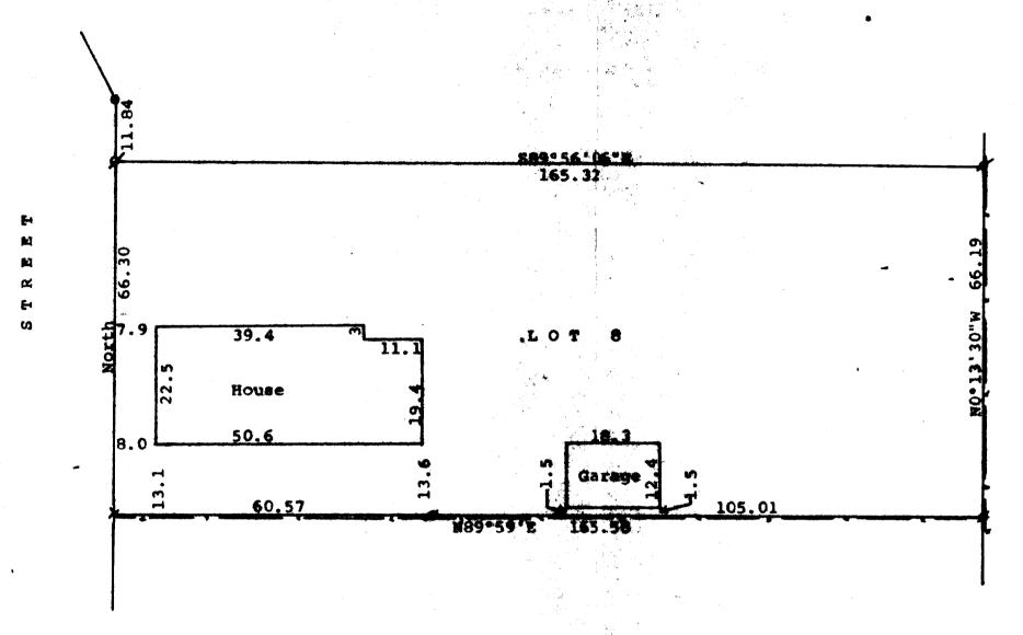
Scale - 1" = 20' ★= found cross in concrete ≠= 3/4" Iron Pipe Found O = 1" Iron Pipe Found
